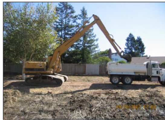
Figure 7. Example of a long-reach excavator that will be used from the north to remove sediment and Ludwigia from Laguna 1 and Laguna 2
